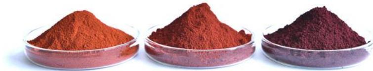
Micronized iron oxide pigments of the proven Bayferrox brand from LANXESS are very easy to disperse and have high color strength and consistency. Because of their property profile, they are mainly used in the manufacture of high-quality paints and coating systems.
