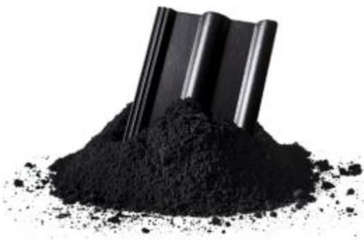
With Bayferrox 303 T, specialty chemicals company LANXESS is offering a unique black pigment for coloring concrete roofing tiles. Compared with conventional black pigments, it reflects 20 percent more of the sun's infrared radiation. Reflective surface materials – especially when used on roofs – can help to counter the urban heat island effect. Photo: LANXESS AG
