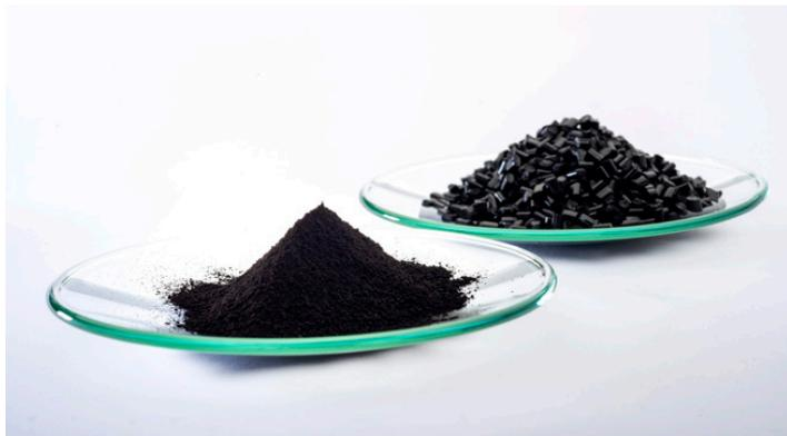
Specialty chemicals company LANXESS has developed a black pigment that reflects 20 percent more of the sun's near-infrared radiation (NIR) than conventional products. By means of coloring with Bayferrox 303 T (in foreground of picture), the service life of plastic components can therefore be extended, as they are less exposed to temperature fluctuations. Photo: LANXESS AG
